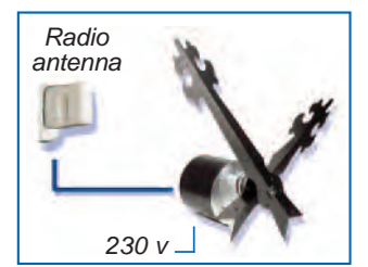
Synchronised by radio or GPS antenna
